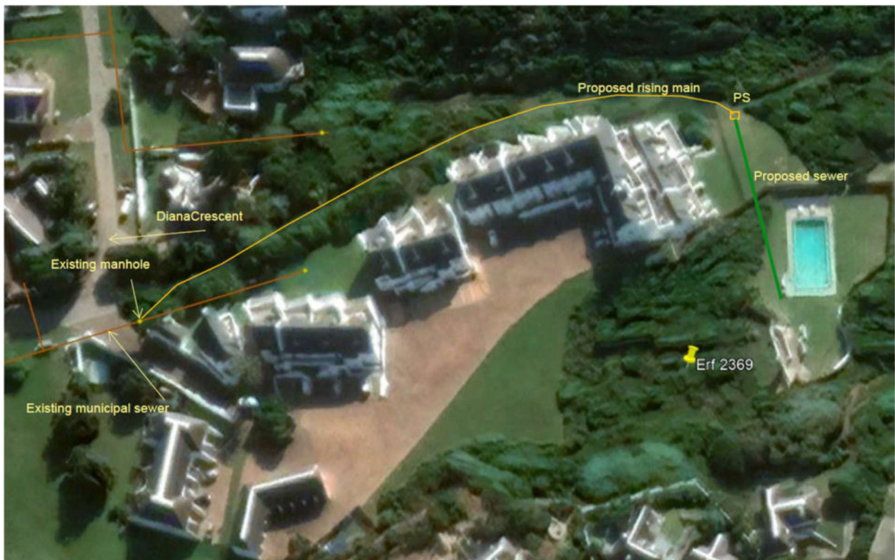
Figure 9: Proposed sewer pump station and rising main
