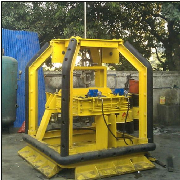
Figure 5-15: Cone penetration test unit
