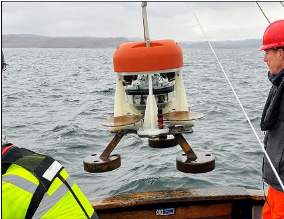
Figure 5-17: Acoustic doppler current profiler buoy
