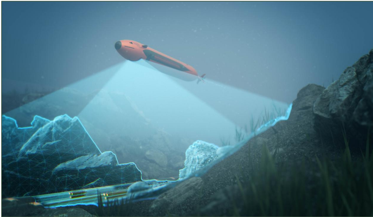
Figure 5-6: Example of a AUV used for bathymetric and sonar surveys
