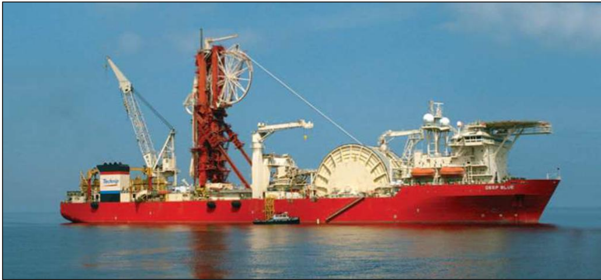
Figure 5-36: Example of deepwater Subsea Construction Vessel (SCV)
